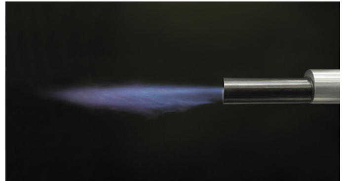
Flame of the ZKIH during natural gas operation in the open air
